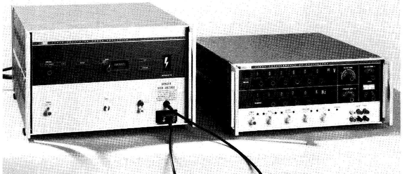
Figure 96. Fluke Models 5200A/5205A Precision AC Calibration Standard. An AC Calibration System Brings To Manufacturing And Laboratory Environments Greater Precision Over Wider Operating Frequencies. The operating AC Frequency Range Should Be 10 Hz to 1.2 MHz And Provide Accurate AC Voltages From 100 \mu V To 1200 Volts RMS.
